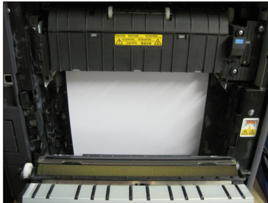
Misfeeds can only be accessed from the rear of the device.
